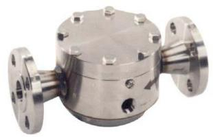
The design of the 140MX does not require a maintained turbulent flow in the pipe for operation. This allows it to be used with **high viscosity fluids** and/or low flow rates. It operates within its specified accuracy at Reynolds Numbers as low as 400 and will continue to provide an output signal at Reynolds Numbers as low as 75. Fluids with Kinematic viscosities up to 80 centistokes can be metered, which provides capabilities for No. 6 fuel oil and other heavy oils.
