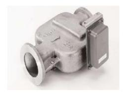
The Model 141 offers a wide operating temperature range for cryogenic applications: -196° to 176° C (-320° F to 350° F), when the optional cryogenic sensor is specified. The Model 141 also offers a wide dynamic range: Reynolds numbers from 10,000 to 1,000,000 and a high turndown (typically 15:1). The design of the meterbody combined with the sensor technology makes the flowmeter highly immune to the effects of sensor buildup or coating.
