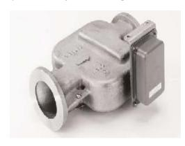
The Model 141 easily handles **low lubricity fluids** such as liquid ammonia. The Model 141 also offers a **wide dynamic range**: Reynolds numbers from 10,000 to 1,000,000 and a high turndown (typically 15:1). The design of the meterbody combined with the sensor technology makes the flowmeter highly immune to the effects of sensor buildup or coating.
